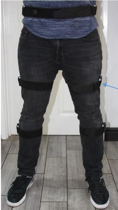
GaitSmart uses six small Inertial Measurement Units (IMUs) mounted on the body using custom straps, at the pelvis, thigh and calf.
